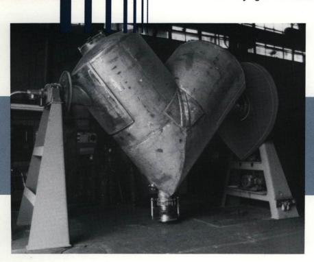
The Rota-Vee is best suited for materials which are "free-flowing" and therefore benefit most from the splitting and rejoining action as the dryer rotates.
