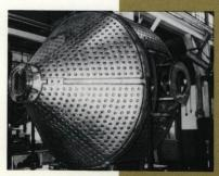
Paul O. Abbe Vacuum Dryers. They can be fabricated from any of the common steels or corrosion-resistant materials. On tumbling vessels jacket designs can range up to 100 psig in the open design to 150 psig for the dimple design. For stationary dryers the jackets can be built up to 200 psig or higher. All pressure jackets above 15 psig are built and stamped per the ASME Code. Jackets are
